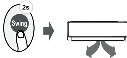
Keep pressing this button more than 2 seconds, the vertical louver swing function is activated. (Model dependent)
