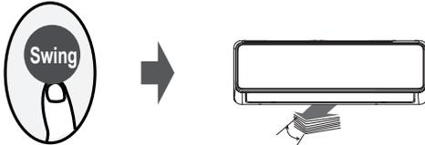
The horizontal louver will swing up and down automatically when pressing Swing button. Press again to make it stop.
