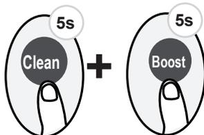
Press together **Clean** button and **Boost** button at the same time more than 5 seconds to activate Lock function. All buttons will not response except pressing these two buttons for two seconds again to disable locking.
