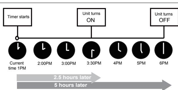
Example: If current timer is 1:00PM, to set the timer as above steps, the unit will turn on 2.5h later (3:30PM) and turn off at 6:00PM.
